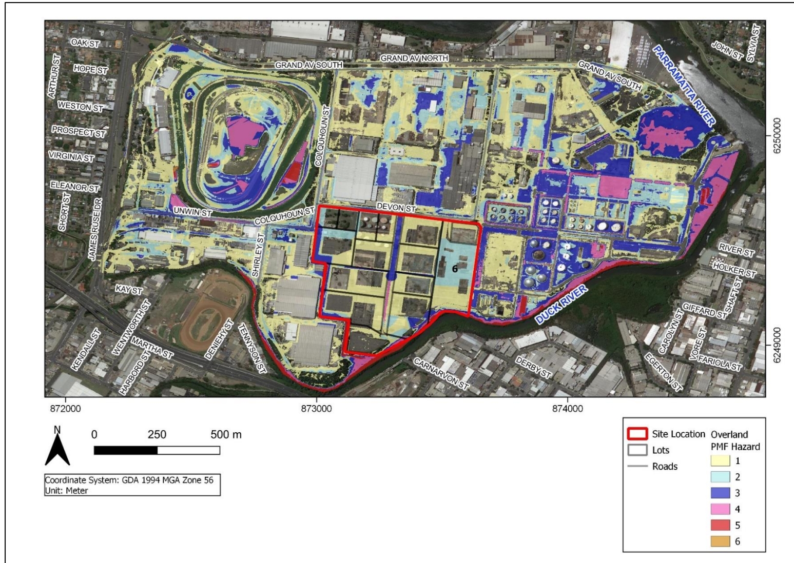
Figure 11. Peak hydraulic hazard for the overland PMF (<5 cm trimmed out).
